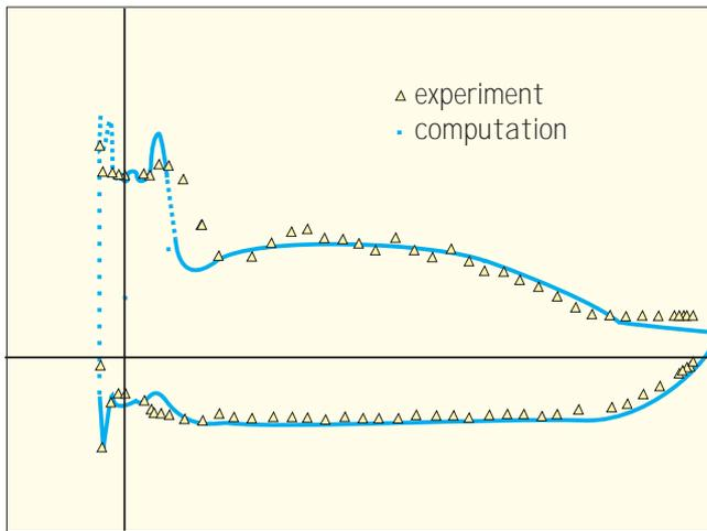
Fig. 6 – Comparison between FLUENT/UNS and experimental 2D pressure distribution around a mast and mainsail geometry
