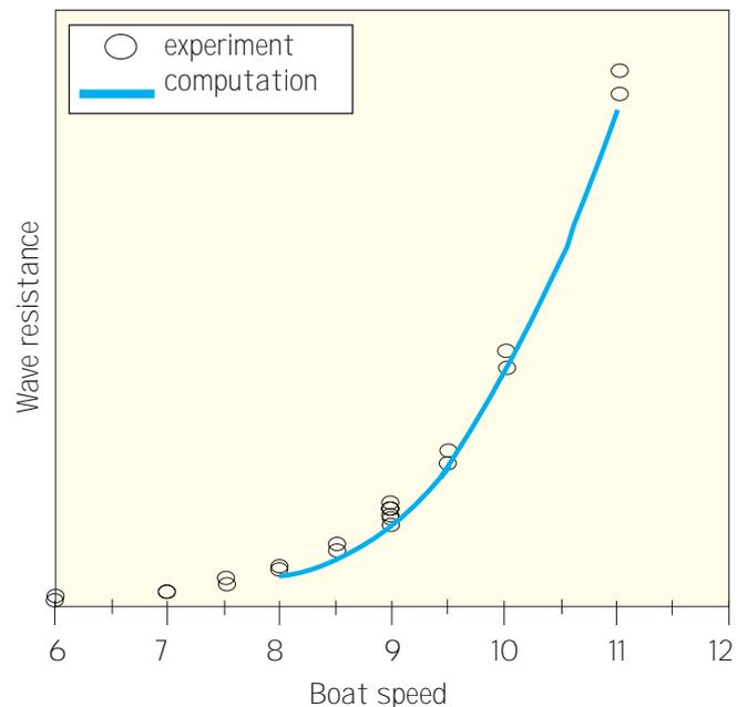
Fig.1 – Wave drag comparison between SHIPFLOW and experimental results
