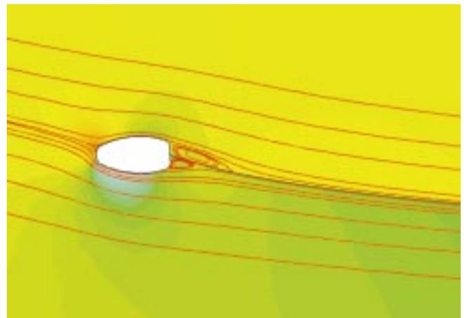
Fig. 5 – Flow around an IACC mast and mainsail geometry computed by FLUENT/UNS
