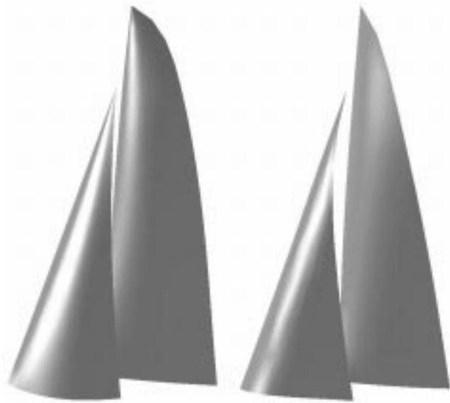
Fig.4 – Design (left) and flying (right) shapes of IACC upwind sails, the latter determined by FLOW-MEMBRAIN aeroelastic computations
