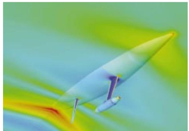
Fig. 3 – Pressure distribution around an IACC hull and appendages computed by FLUENT/UNS
