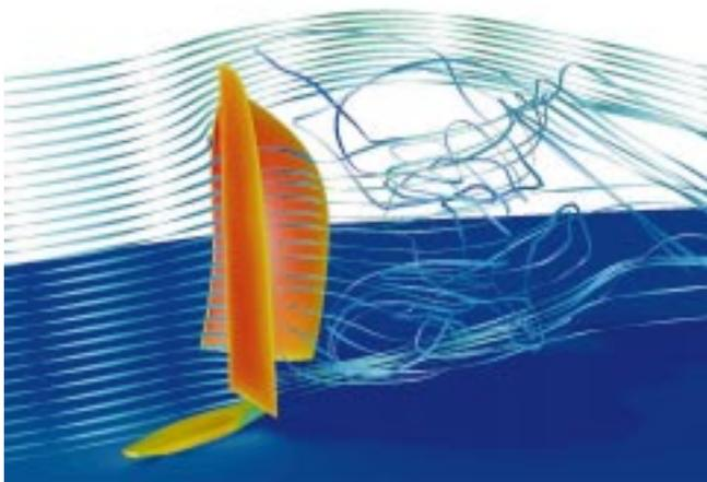
Fig. 7. – Surface pressure contours and streamlines for flow around a downwind sail configuration of an IACC yacht computed by FLUENT/UNS
